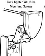
Re-position the transducer assembly against the transom of the boat, then hand-install all three screws. Make sure that the transducer location and the pivot angle have not changed, then fully tighten all three mounting screws. Snap the pivot back down. If you have performed the preceding procedures correctly, the transducer should be level and at the right height for optimal operation.
